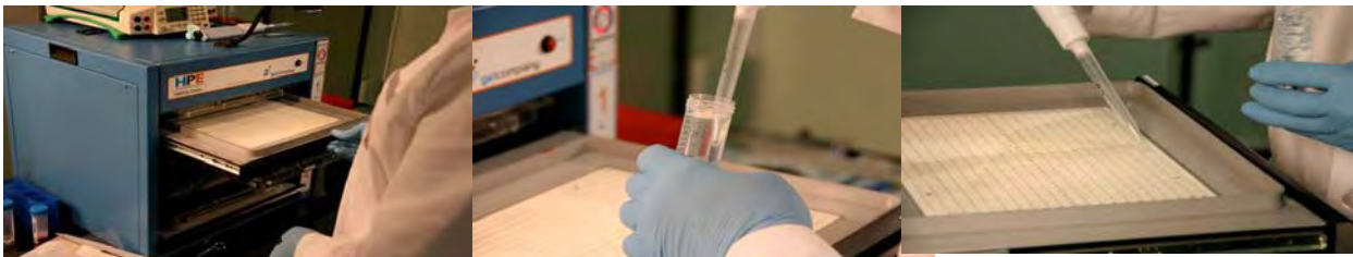
Fig. 5.3: Application of the cooling fluid
