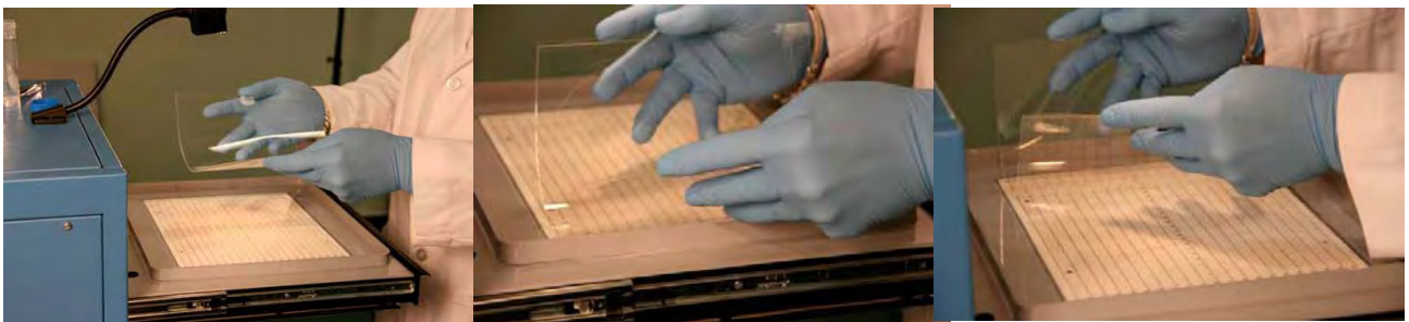
Fig. 5.4: Placing the gel on the cooling plate; distribute the cooling fluid evenly.
